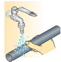
Figure X-b – Clean Pipe Ends
