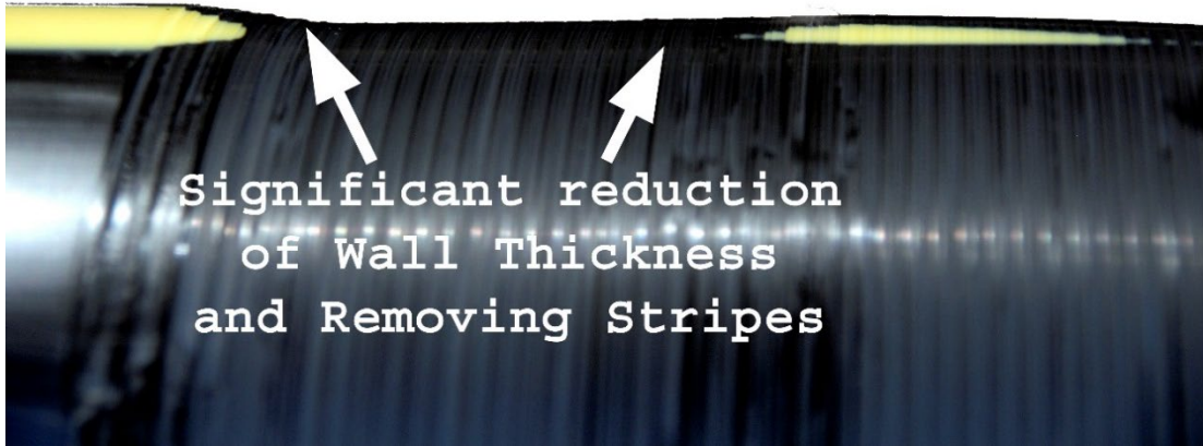
Over Scrape Unacceptable Possible Causes: Incorrect Scraper, Poorly Maintained Scraper, Excessive Number of Passes With Scraper, or Ineffective Evaluation of Scraping
