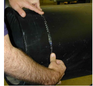
Figure IV-a - Measuring pipe diameter with Pi tape
