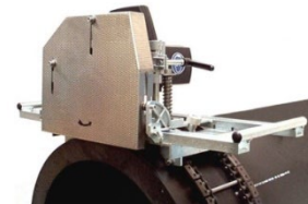
Figure X-a – Cut Pipe Ends
