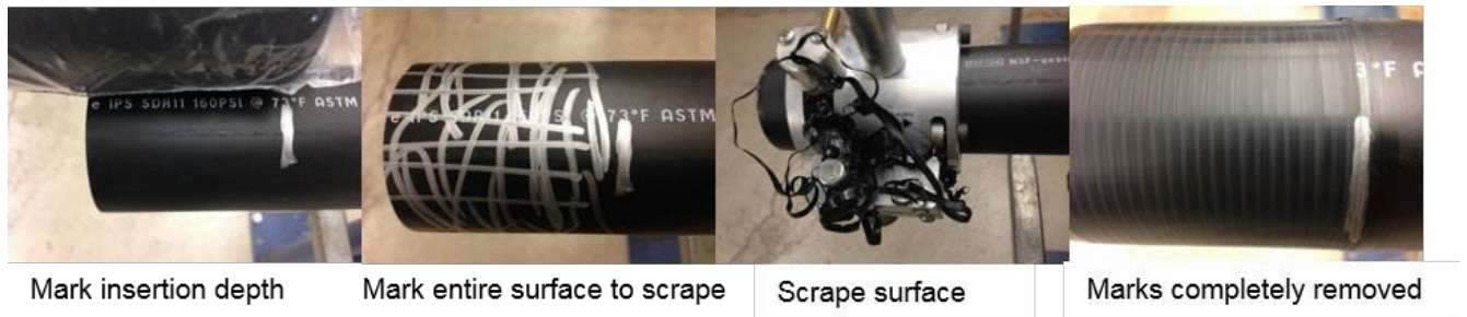
Figure X-r - Correct Scraping
