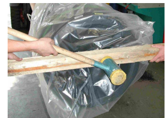
Figure X-g – Avoid Contamination During Installation
